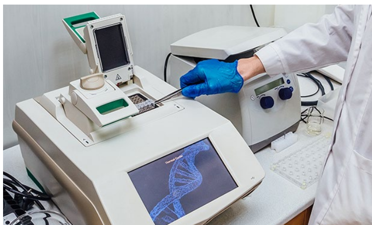
Image of a scientist with gloved hand putting DNA sample into real-time PCR-cycler.
